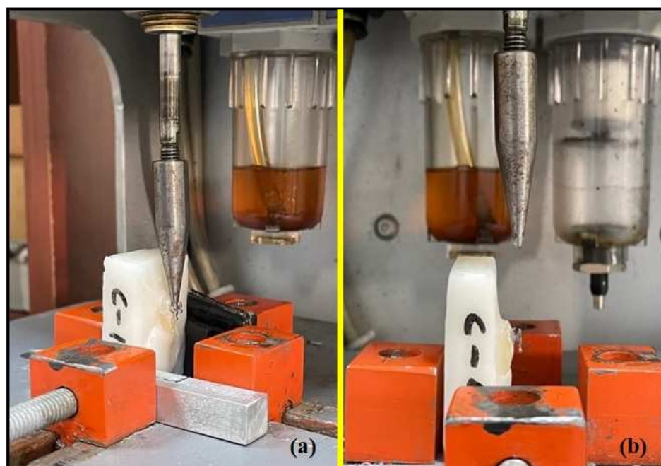
Figure 3. Checking the angle between the bracket groove and the metal nozzle tip from the lateral (a) and from the frontal (b).
