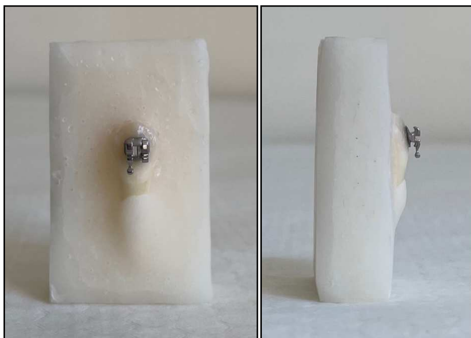
Figure 1. The buccal surfaces of the teeth are embedded perpendicular to the stainless-steel nozzle tip, which will exert the shear force.
